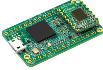
Figure 6.3: *BGT60TR13* Radar System. The radar sensor, is mounted on top of the board.
