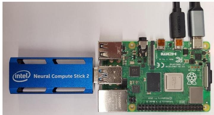
Figure 6.7: Recording setup for the offline proof-of-concept of the system generalization capability at the edge. The Raspberry<sup>®</sup> Pi4 is used for data preprocessing, model adaptation and script running. The NCS 2 enables the deployment of the developed meta-learning model for a specific setup.
