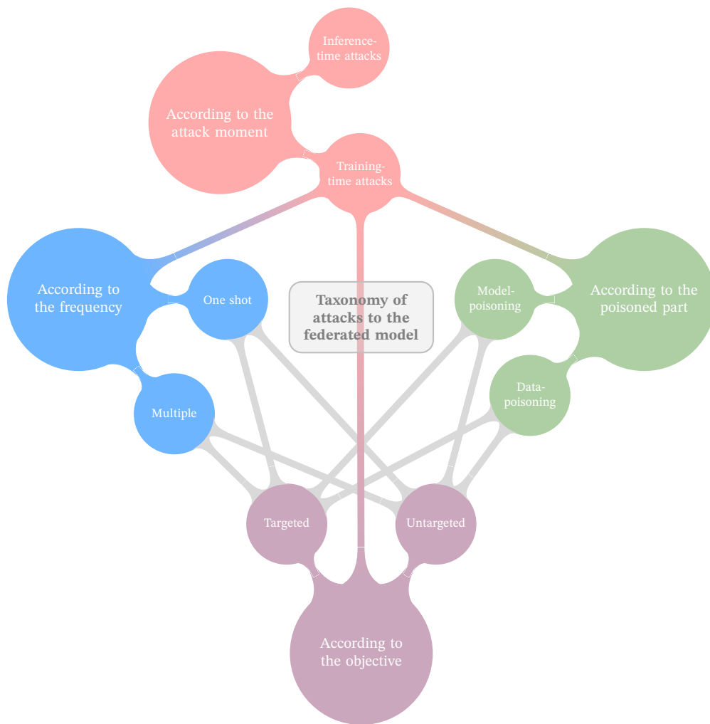
Figure 3: Representation of the attack taxonomies to the federated model according to the different criteria. The grey links represent the possibility of combination of both categories. For the sake of clarity, we don't show redundant connections between categories already connected with other links.
