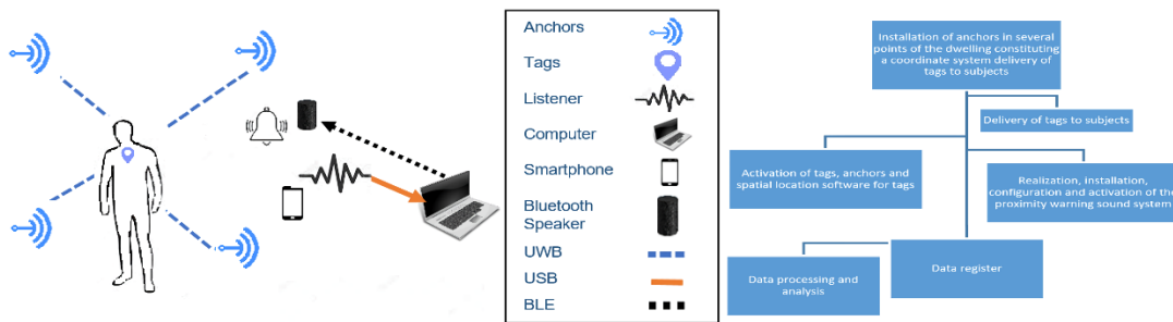
Figure 2. Scheme of the system and devices.
