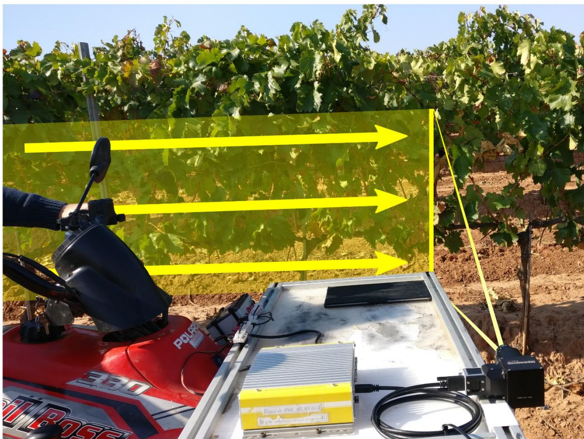
572 Fig 2 On-the-go hyperspectral imaging with a camera mounted on an ATV at 5 km/h. Images of the 573 entire vine canopy were obtained from the ATV's motion, by push-broom scanning, and used for the 574 estimation of grape composition.
