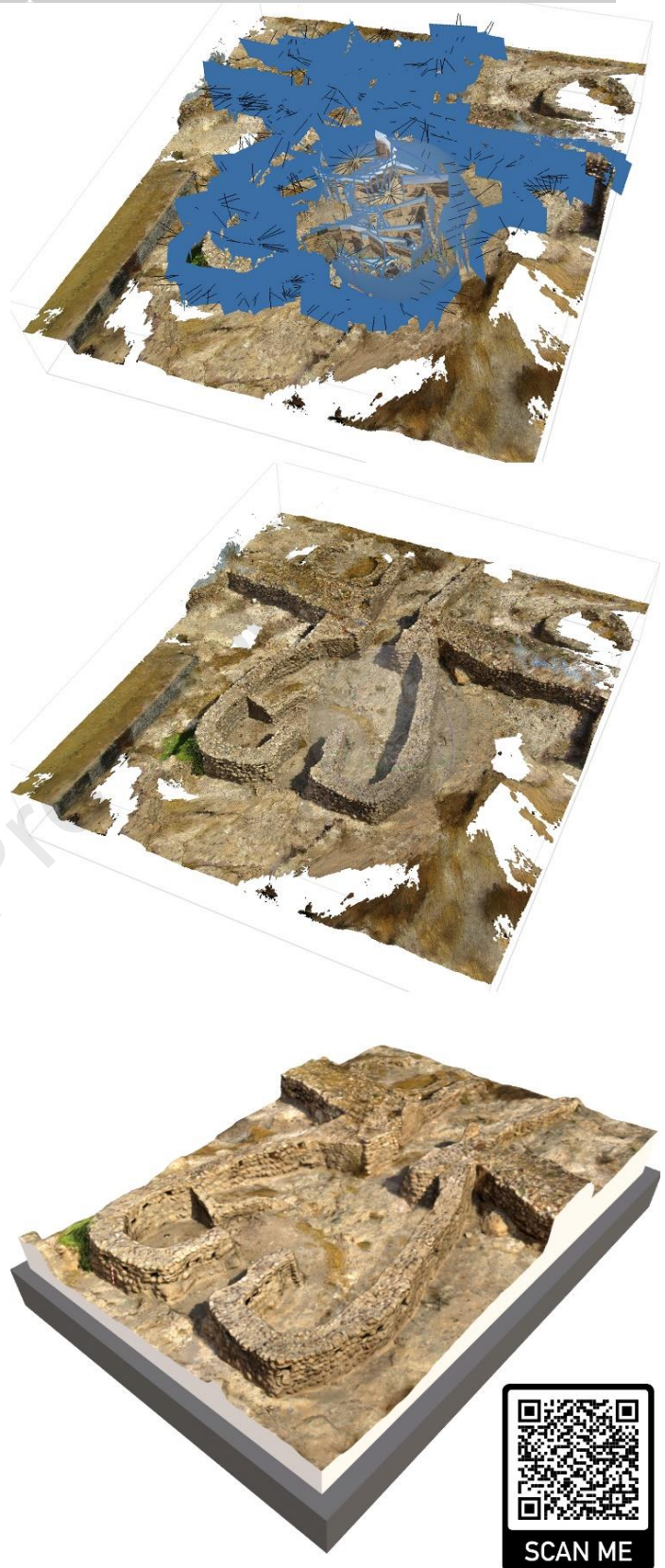
Figure 10. Processing the photogrammetric model of the barbican in Agisoft Metashape. The first two models show different stages of its processing, and the last one is the final model. Note the QR code attached to the image.
