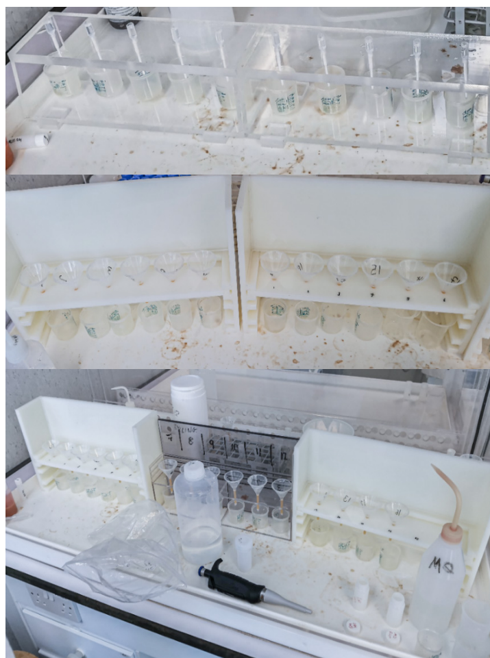
Figure A3. The setting of cation exchange columns in a clean laboratory.
