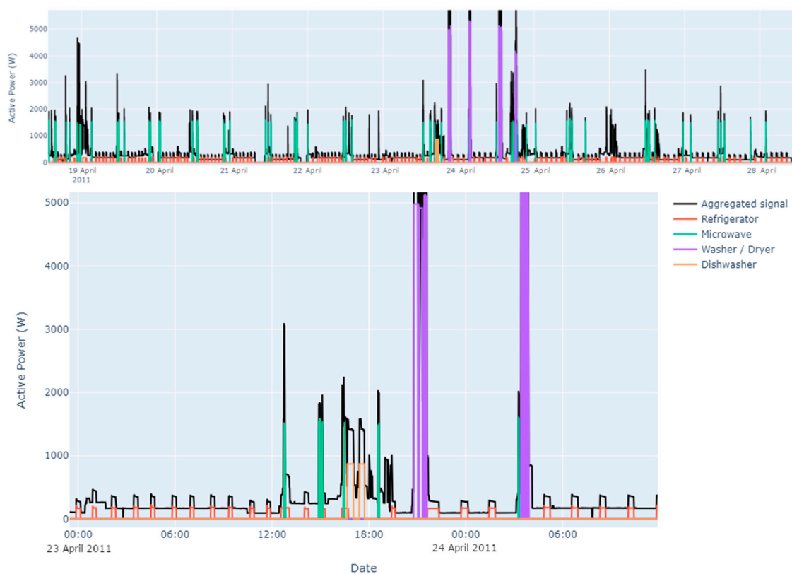
Figure 7. Appliance disaggregation in the first two weeks of REDD House 1 with a zoomed-in version for 23 April 2011.
