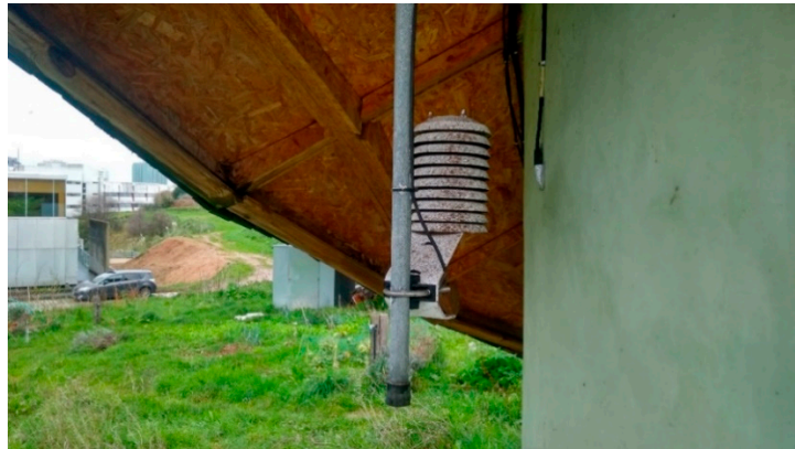
Figure 2. Temperature probe of the case study.
