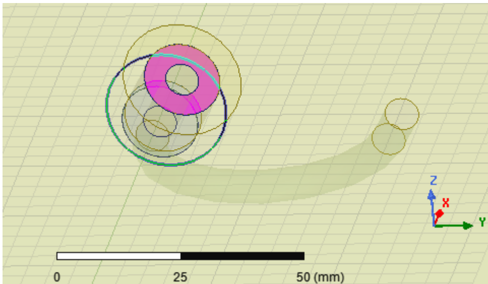
Figure 3.23 – Example of excitation selection in HFSS
