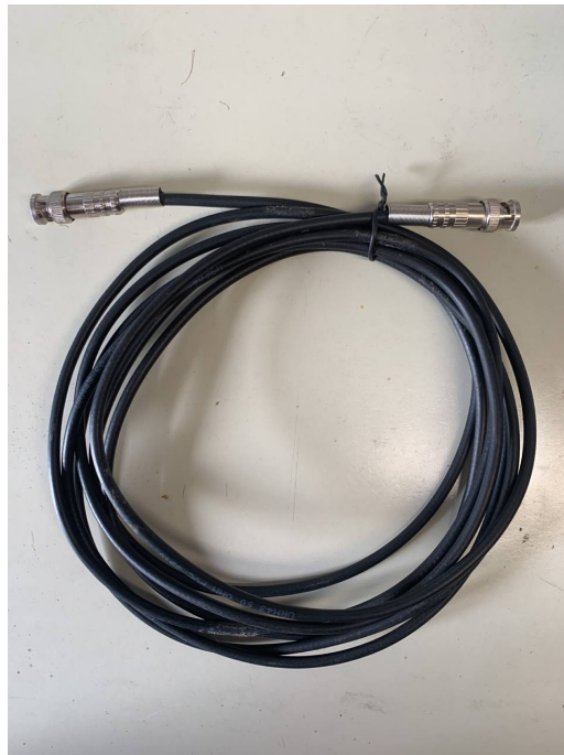
Figure D.7 – Finished male BNC pigtail
