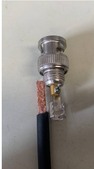
Figure D.2 – Outer dielectric stripped
