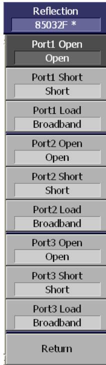
Figure A.4 – Reflection calibration
