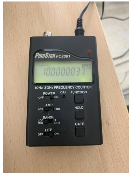
Figure C.3 – FC2001 frequency measure on the XSRM output signal
