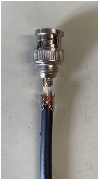
Figure D.5 – BNC connector before tightening
