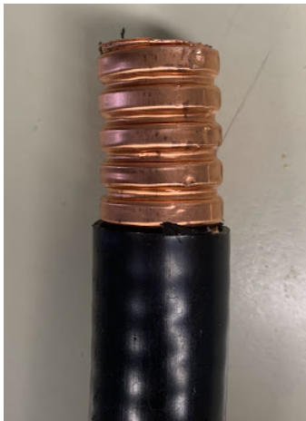
Figure B.1 – Outer dielectric cut off
