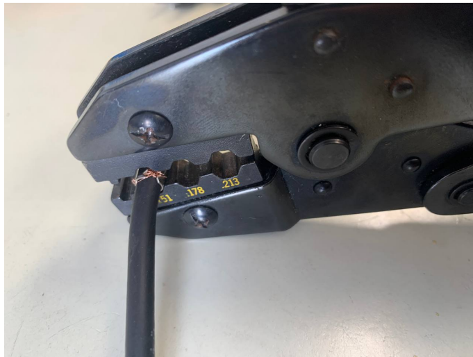
Figure D.6 – BNC connector crimping
