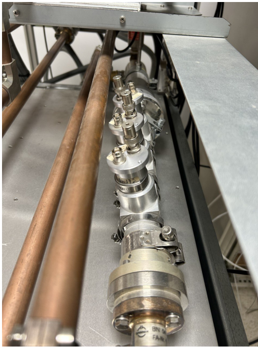
(a) Before load directional couplers
