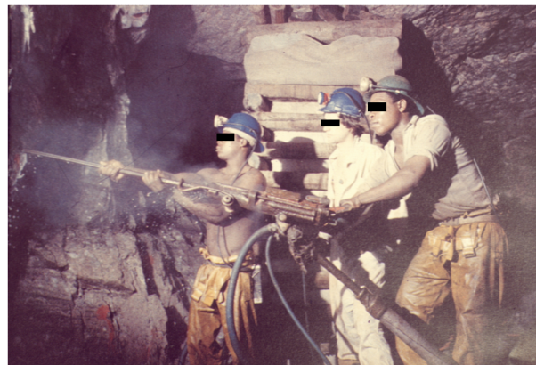
FIGURE 2 Rock drill operators in a gold mine. Source: Centre for Environmental and Occupational Health Research, University of Cape Town (reproduced with permission)
