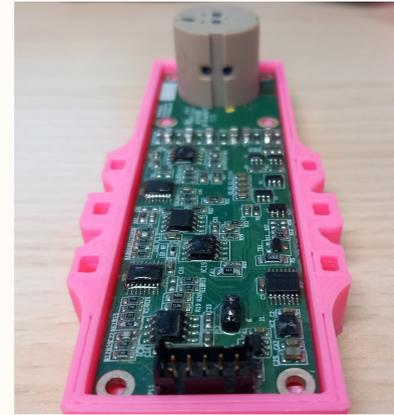
The Mag651 is a sensor consisting of a cluster of three feedback stabilised, fluxgate sensors arranged along X, Y and Z axes. Each axis provides a highly linear magnetic response with low hysteresis, and low crosstalk between axes.
