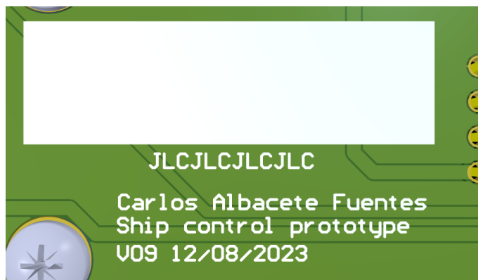
Figure 5.35 – PCB info, blank rectangle and order number indication
