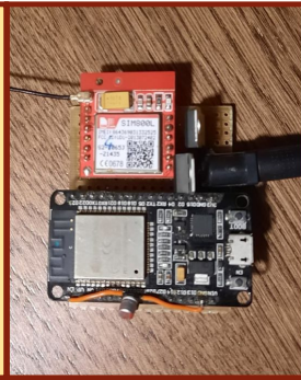
SIM800L test circuit
