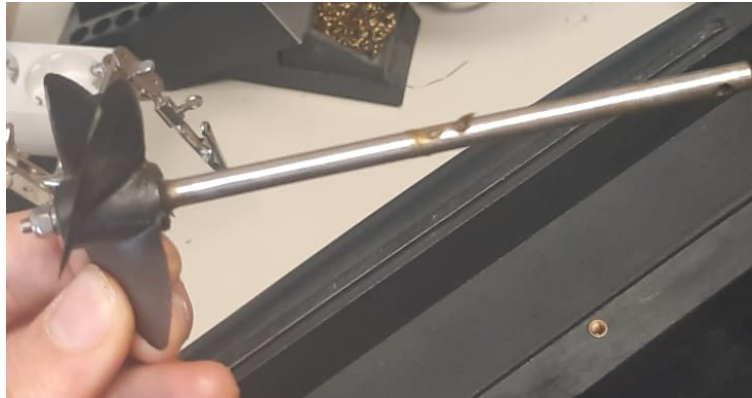
Figure 3.17 – Boat's propeller and drive shaft
