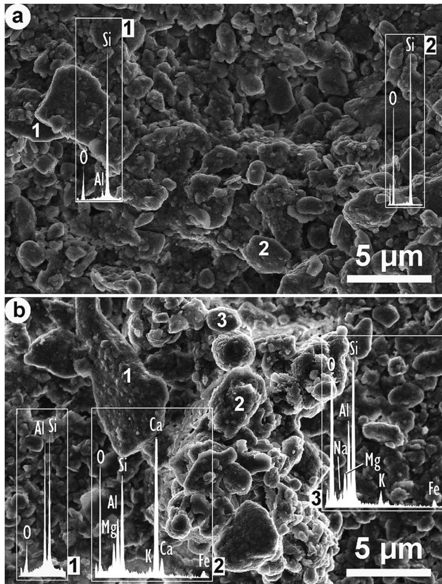
**Fig. 3.** Sample LLB15 (March 2022). An example selected from the red rain samples collection. Dust-borne particles of different size and chemical (mineralogical) composition. General roundness of particles edges can be seen (aeolian modelling). The agglomerated and stratified aspect is due to the preparation technique. a) Field of particles with an average size of 1.17  $\mu\text{m}$  (0.18–4.91  $\mu\text{m}$ ). Chemical composition: 1. EDX, Si, O (Quartz) 2. EDX, Si, O (Quartz).
