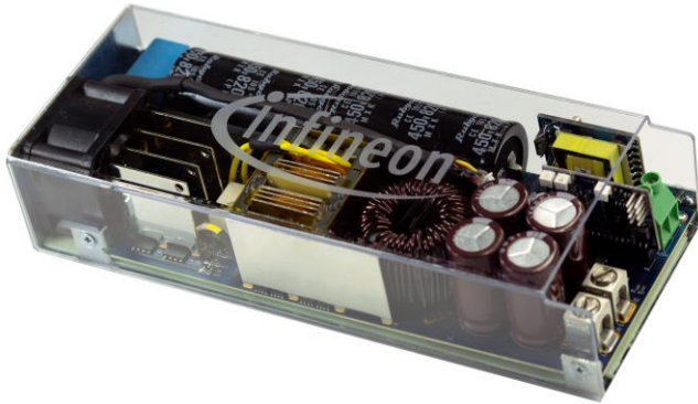
Fig. 16. Prototype of the 3300 W PSFB converter.
