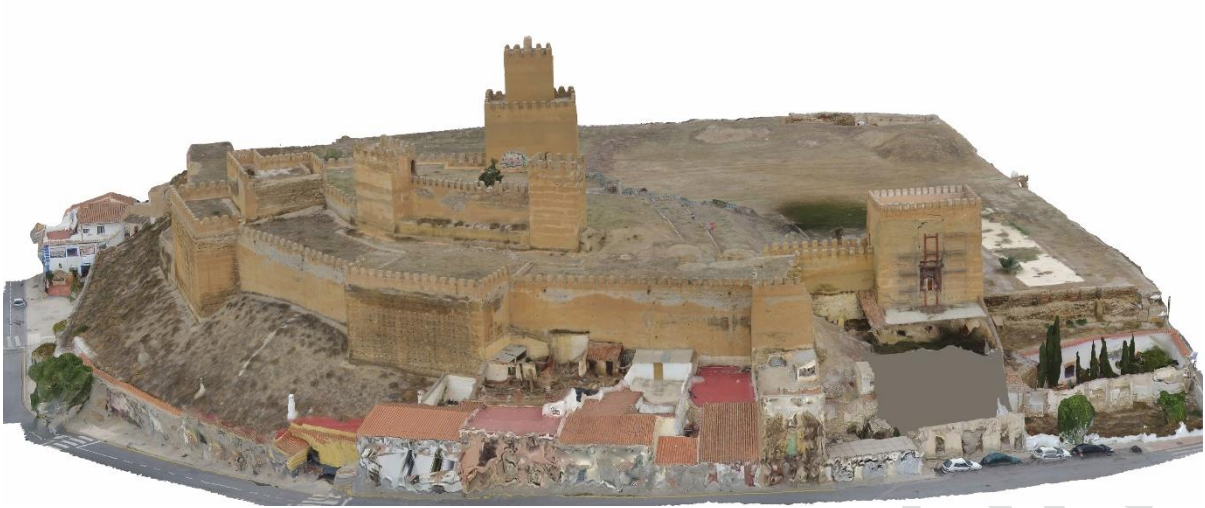
Figure 7. 3D model of the Alcazaba and its surroundings based on a cloud point (44,875,872 points). View from the south. J. A. Benavides López.
