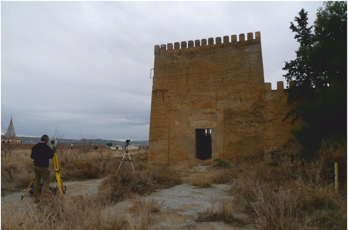
Figure 3. Surveying the topographic points of the Alcazaba of Guadix. J. A. Benavides López.
