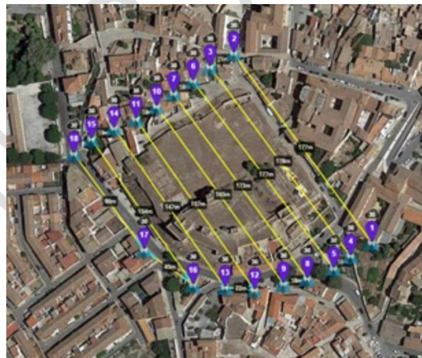
Figure 4. Aerial view of the Alcazaba with the position of the parallel trajectories programmed for the Unmanned Aerial Vehicle (UAV) by the Litchi app for Android https://flylitchi.com . J. A. Benavides López.
