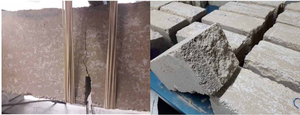
Fig. 11. Specimen A1. Detail of the fracture zone (left) and interior of the material after the test (right).
