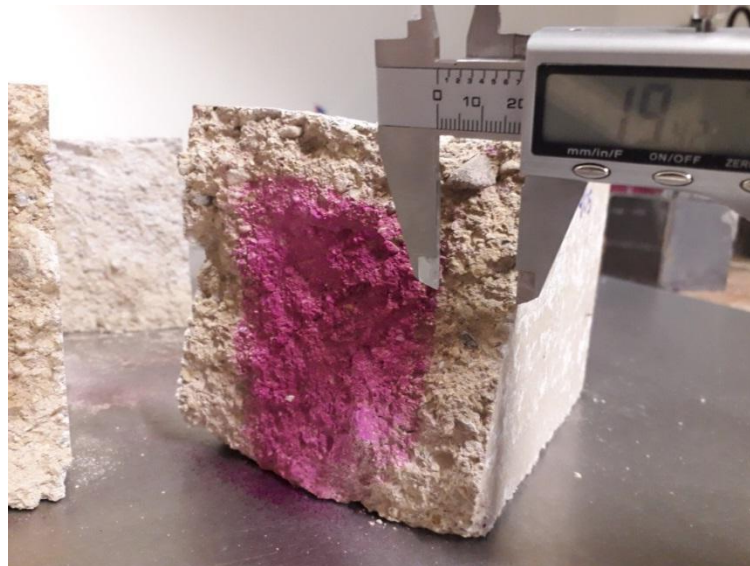
Fig. 8. Carbonation front measured on the control specimen at 48 days (19.42 mm).
