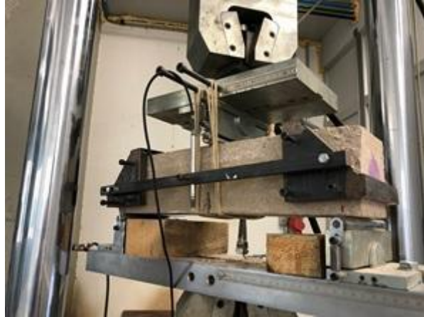
9 10 11 12 13 14 15 16 17 18 19 20 21 22 23 24 25 Fig. 4. Three-point bending test of the specimens. 26 27
