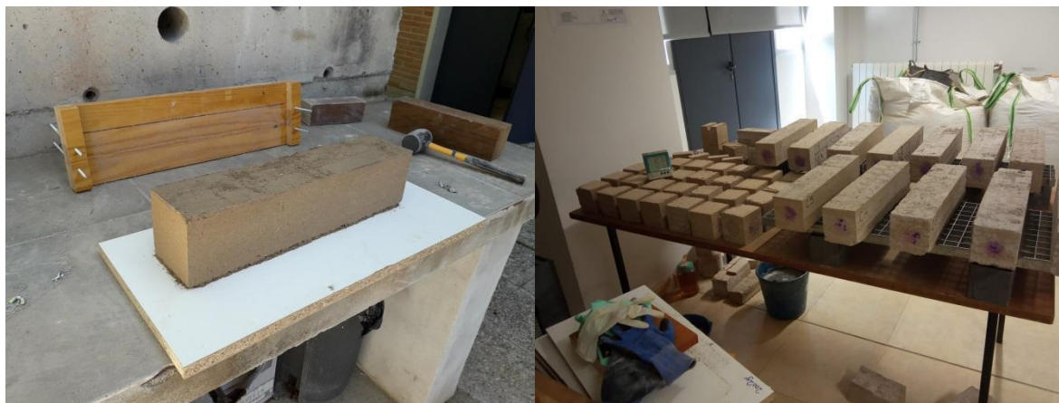
Fig. 2. Production of specimens (left) and storage and curing process in the laboratory (right).
