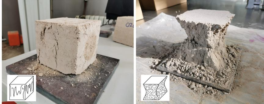
Figure 4: Satisfactory failures of cubic specimens, according to EN 12390-3 [52].
