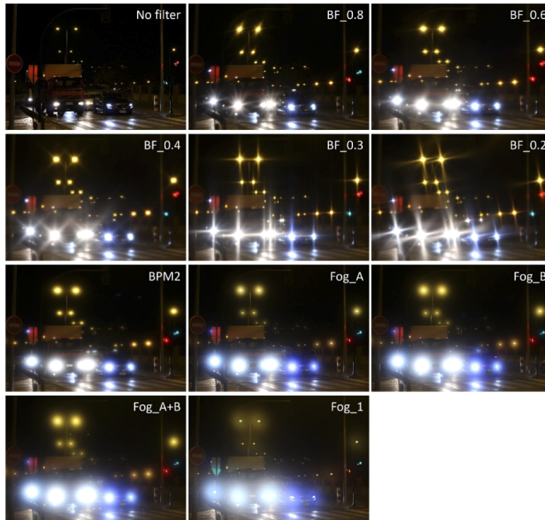
Fig. 1. Night traffic scene with no filter, and as perceived through each filter/foil studied. Each image corresponds to a photograph taken by a commercial camera (Canon EOS 650D) with no filter and using each of the filters/foils analyzed for a fixed configuration of the camera ( f/5.6 ; 1/30 s; ISO 800, 40 mm).
