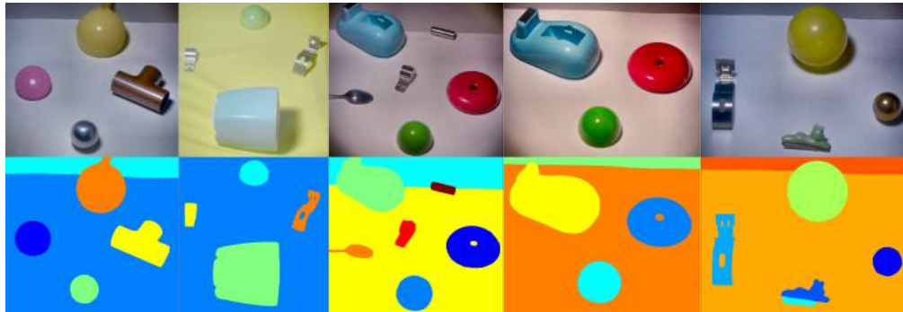
Fig. 10. Top row: RGB renderization of original spectral cubes. Bottom row: benchmark manually segmented. From left to right, scenes from 1 to 5.
