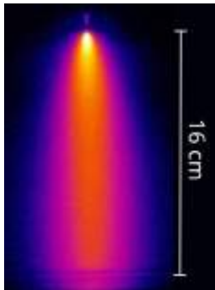
Figure 1.3: A diffuse glow discharge in air at 25 hPa from a positively charged electrode at the top given a pulse of 14.6 kV with 15 ns rise time and 10 \mu s decay time. The photograph extracted from Nijdam et al. [703, fig. 5], was exposed for about 2 \mu s.
