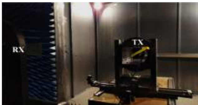
FIGURE 10. Measurement scenario for the SISO system inside the reverberation chamber. A transmitter antenna (TX) points at the metallic wall of the chamber and a receiver antenna (RX) acquires the multiple reflections inside it.
