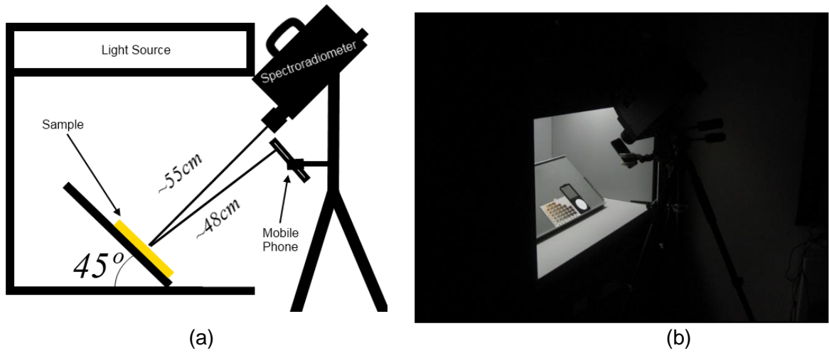
Figure 2: (a) Scheme of the measurement process. (b) Photograph of the experimental setup during the calibration process (the reference white is placed at the right of each Munsell Hue chart containing chips with different Value and Chroma).
