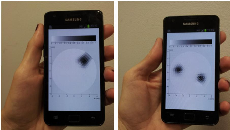
Fig. 7. Developed Android application used for image reconstruction.
