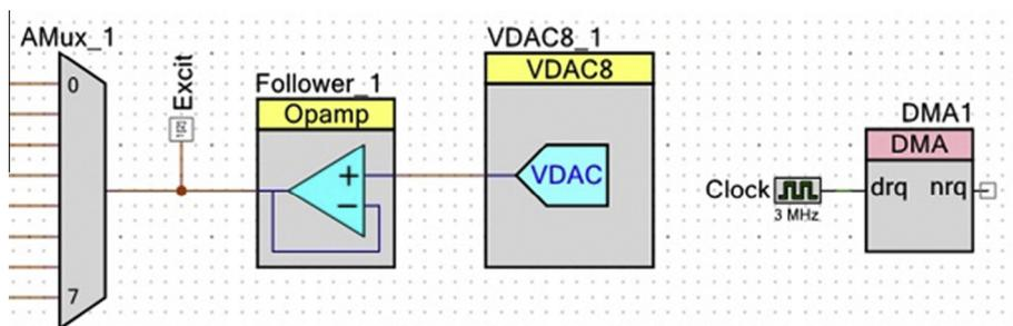
Fig. 2. Generation of the excitation signal.
