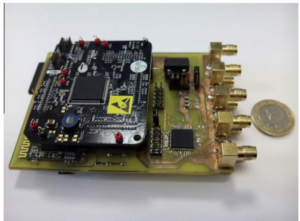
Fig. 4. PSoC-based integrated system for ECT.
