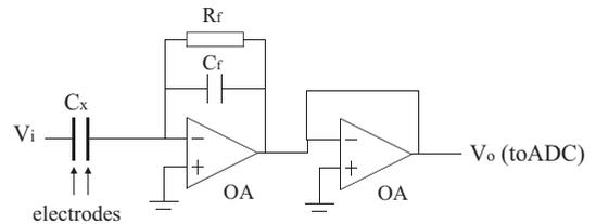
Fig. 3. Analog blocks arrangement for capacitance measuring.
