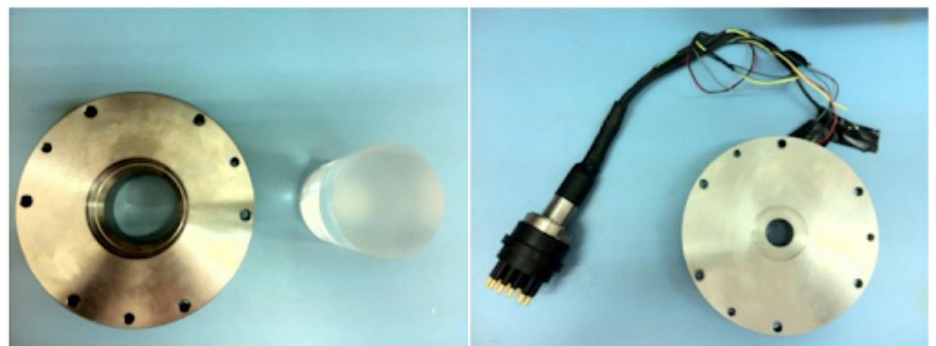
Figure 7. (Left) Glass rod next to the top cap where it is inserted. (Right) Bottom cap with the connector of the laser beacon.
