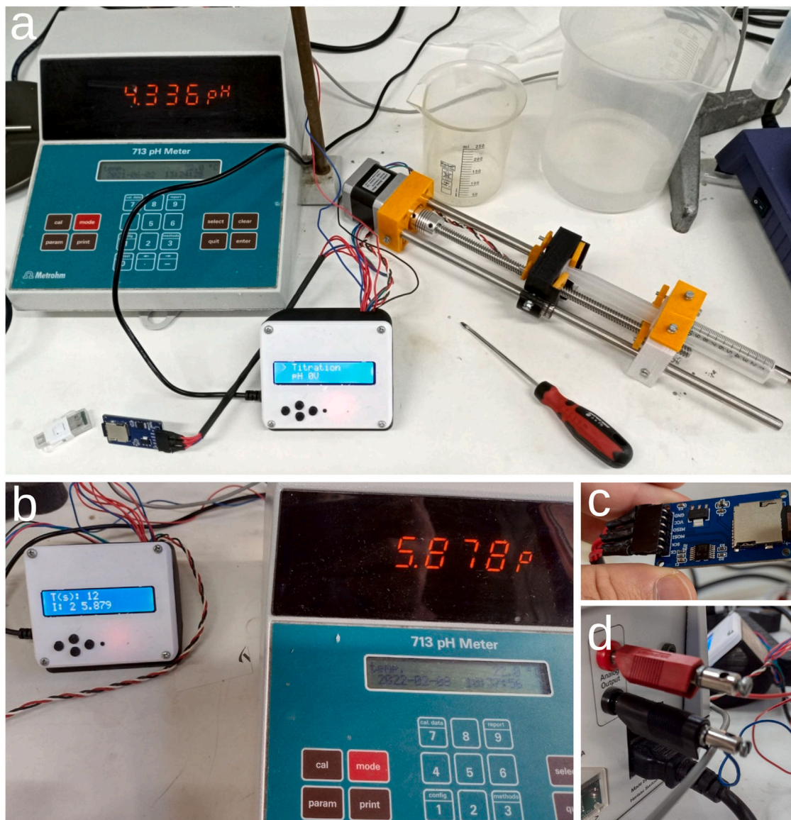
Fig. 5. (a) OSPump Titrator based on Arduino [7]. (b) Detail showing a titration where the reading in the left LCD panel corresponds to the measurement from the Metrohm 713 pH meter on the right. (c) MicroSD card module to store the data of the quantity of NaOH solution pumped to keep a constant pH in the sample, keeping track of the pH and added volume over time. (d) Analog output from the pH meter used as input for the OSPump Titrator.
