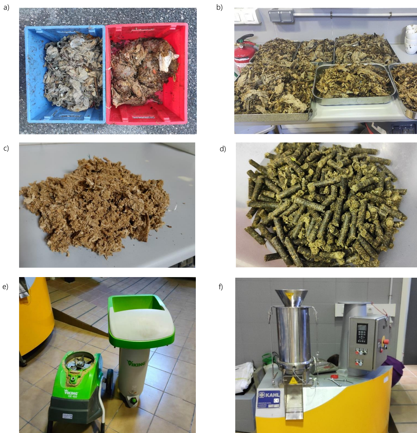
Figure 21. Non-densified and densified Solid Recovered Fuel (SRF) production process. a) Waste after collection. b) Dry waste. c) Non-densified SRF. d) Densified SRF. e) Bio shredder Viking GE450. f) KAHL 14-175 Pelletizer
