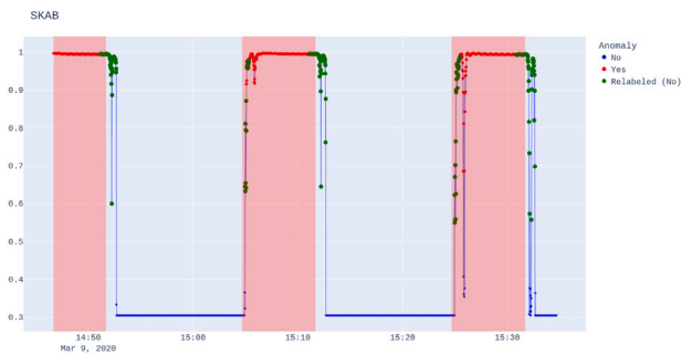
(a) Plot of the results of applying the XGBOOST algorithm in the FP mitigation stage from the WeiXiaoYan results.
