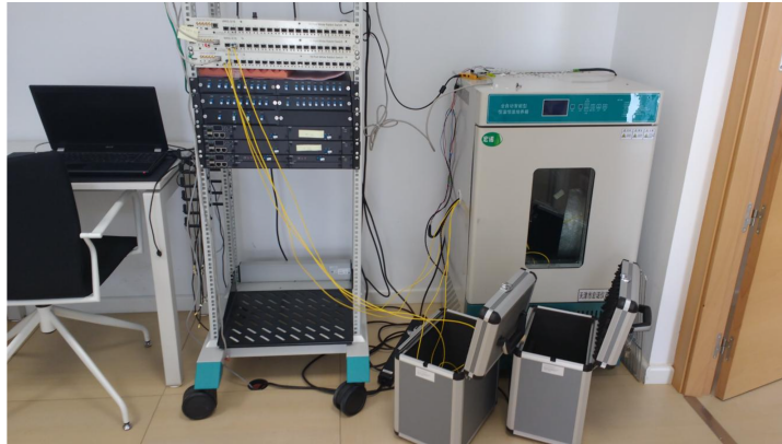
Figure 5.8: Long distance testbench. Three WRS are shown on top of the rack, and MUX/DEMUX devices, OADM, EDFAs and DCMs follow from top to bottom. Spools of fiber are contained in the grey metal cases, and the device in the right side corner is a climate chamber that allows us to establish a precise temperature of operation.
