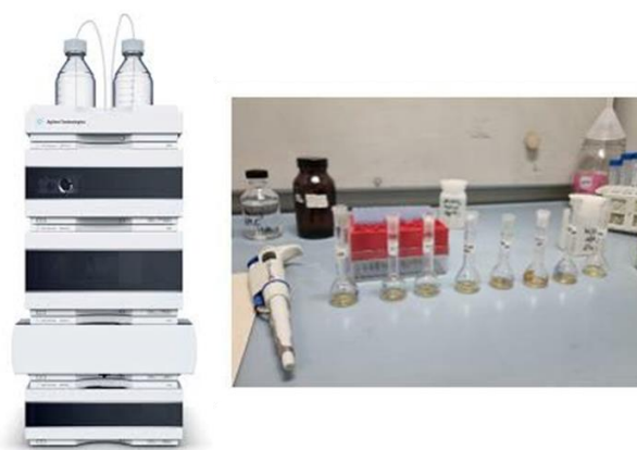
Figure 3.2: Biogenic amines quantification through HPLC injection.
