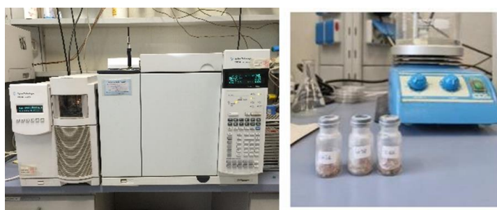
Figure 3.3: Volatile organic compounds analysis through GC-MS-SPME technique.
