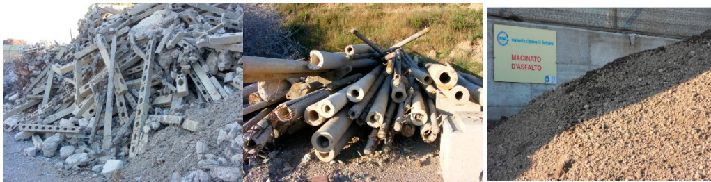
Figure 6. Examples of properly managed CDW materials, deriving from selective demolitions (from the left: concrete structural elements, mixed materials from water systems, and finally, ready-to-use ground asphalt from road pavement demolition).
