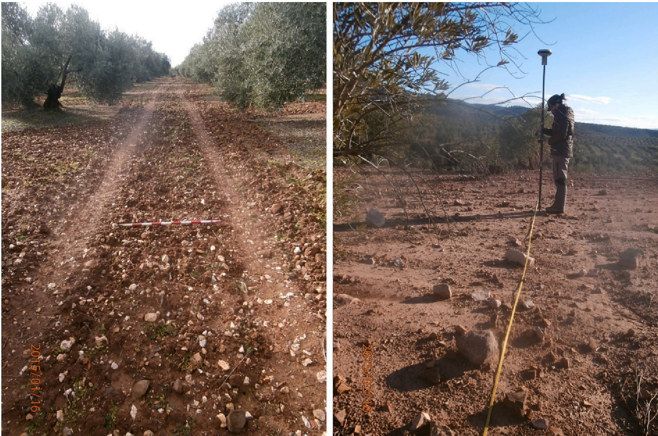
Fig. 4. La Florina. Aluminium range rod on the impressions made by a tractor (left part). Llanos de Vichi. Surveying a transect with GPS and measuring tape (right part).
