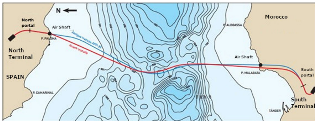
Figure 1. Tunnel layout proposal. Red line shows new proposal whereas blue one shows previous one.
