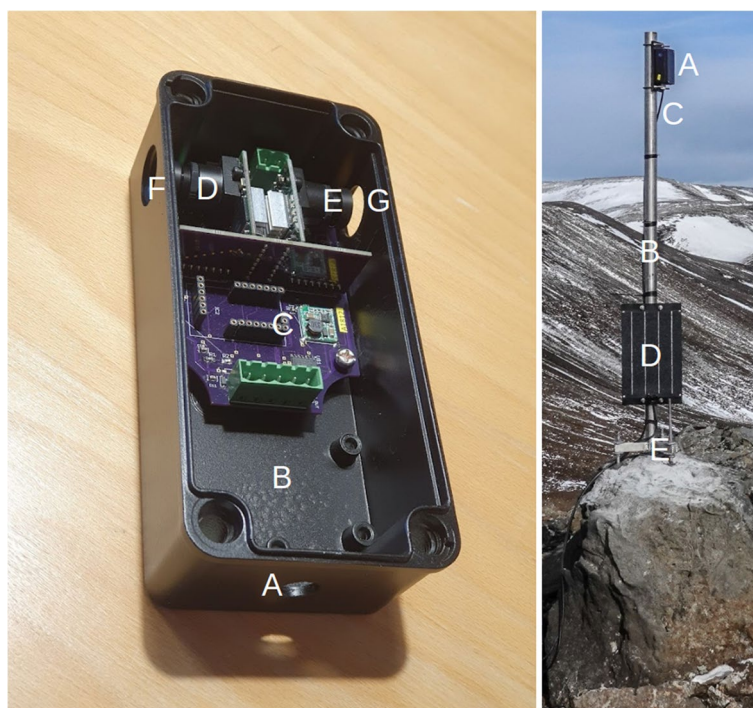
Fig. 2 Left: A disassembled ArduinoCam unit. (A) aperture in the weather proof box for the power cable, which powers the modem which transmits images over the cell network (located in the space (B) ) and the Arduino single board computer (C) . Two cameras are connected to the Arduino (D, E) with views in opposite directions through windows cut into the box (F, G) . Right: An example ArduinoCam installation at Slaga for monitoring the Fagradalsfjall eruption. The unit (A) is mounted on a steel pole (B) , which guides the power cable (C) down to a 12V battery that is charged by a solar panel (D) . The steel pole is bolted to a stable rock (E)
