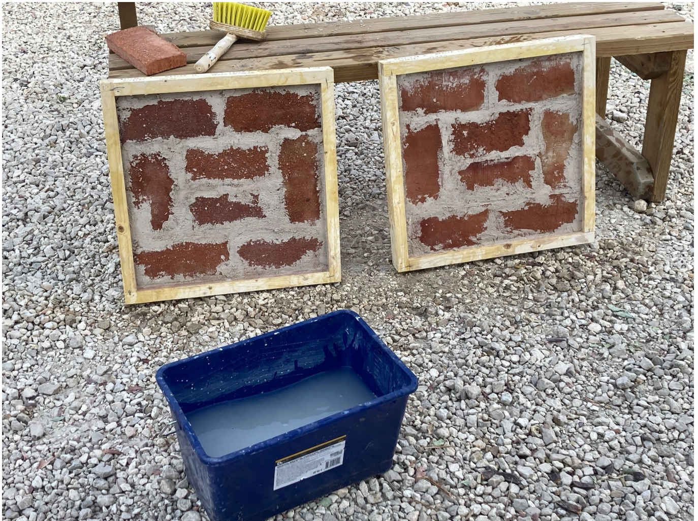
Figure 2. Water applied to 'rustic' brick before they are plastered with opus signinum , during the 2021 opus signinum recreations of the AQUAROLE project, at the Lime Museum of Morón (Seville). Image by the author.
