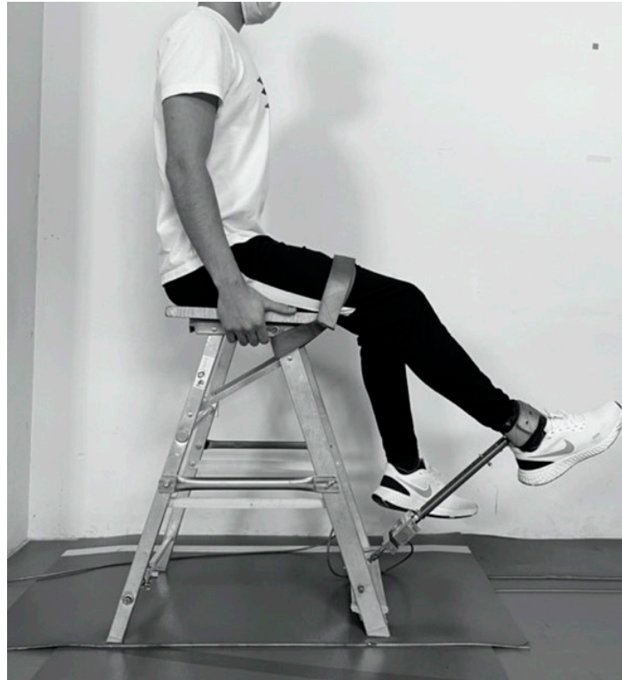
Figure 1. Image of the custom-built bench, placement of the portable strain gauge and participant's position for the measurement of hamstring and quadriceps strength using a field-based test.
