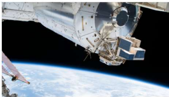
Figure 4. Real image of the ASIM module on the Columbus External Payloads Adaptor (CEPA) of the ISS.
