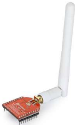
Fig. 5: Transceptor LoRa y antena LoRa BEE.
