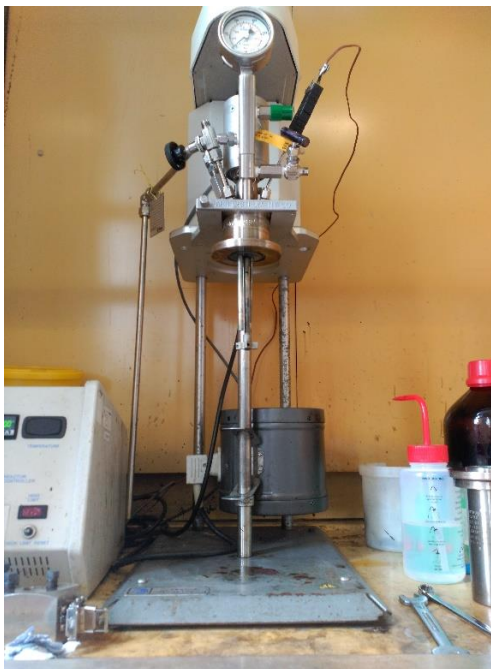
Figure 15. Image of the stainless-steel Parr reactor series 4590 used for the experiments
