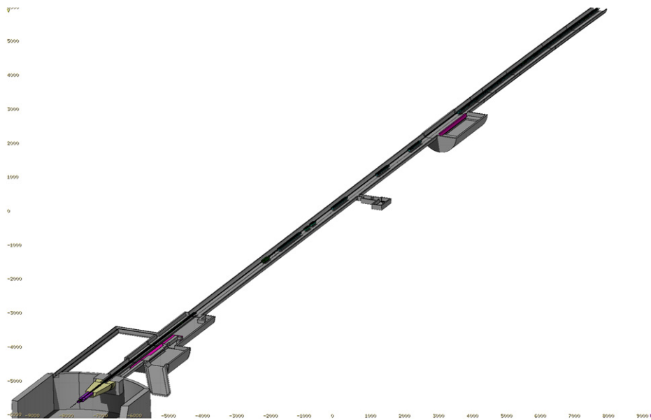
Figure 24. View of a portion of the FLUKA model of the HL-LHC. On the bottom left, one can see the ATLAS forward shielding surrounding the TAXS. The LHC tunnel extends to the west of the ATLAS IP up to the first DS cells (top right), with the violet wall shielding the RR alcove that sits at 250 m from the ATLAS IP.
