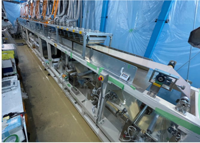
Figure 55. The emulsion film coating system.
