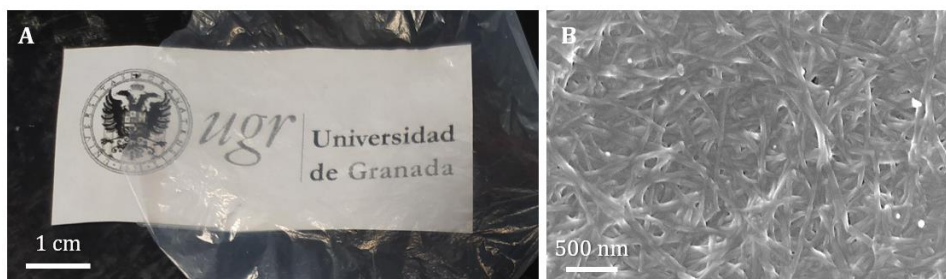
Figure 8. (A) Static pure BC after drying at RT. This drying technique leads to films with higher density than aerogels, almost transparent appearance, and a more compact microstructure, as shown in FESEM micrograph (B).
