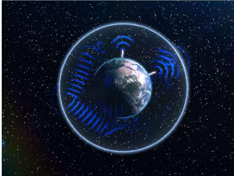
Figure 1.1. Illustration of the Earth-ionosphere cavity, and the SRs generated by lightning activity. The scheme is not scaled. From NASA, 2013. https://www.nasa.gov/mission_pages/sunearth/news/gallery/schumann-resonance.html .
