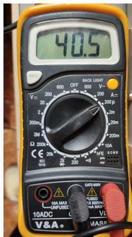
Figure 3.3 – Measured battery charge current
