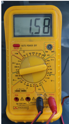
Figure 3.2 – Measured battery voltage
