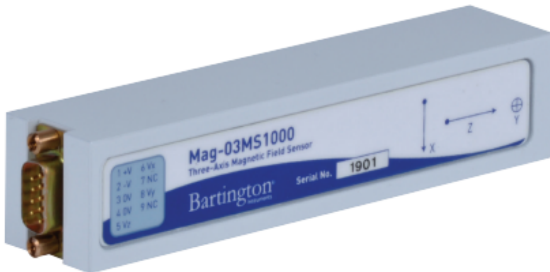
Figure 20: Image of the Mag03-MS1000 magnetometer used.
