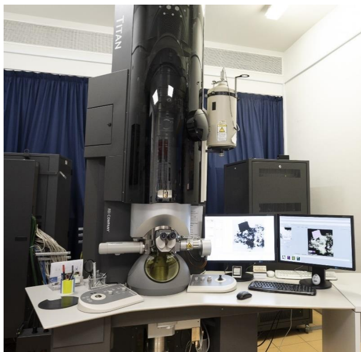
Figure 5. High-Angle Annular Dark Field Scanning Transmission Electron Microscope FEI TITAN G2 80-300 available at Centro de Instrumentación Científica (Universidad de Granada) .
