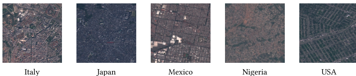
Figure 4.1: Illustration from different countries of the Sentinel-2 satellite images corresponding to one of the 29 Land-Use and Land-Cover (LULC) classes (e.g. Urban and built-up area) extracted from Sentinel2GlobalLULC dataset. Each image has 224 \times 224 pixels of 10 \times 10 m resolution. Pixel values were calculated as the 25th-percentile of all images captured between June 2015 and October 2020 that were not tagged as cloudy. Fifteen LULC products available in GEE agreed in annotating each image to represent one LULC class
