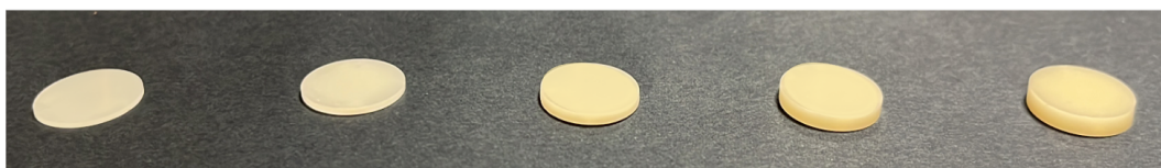
Figure 3.2: Finished VD specimens after polymerization and polishing.
