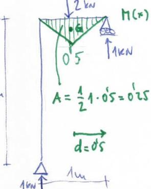
$$\begin{aligned} \delta H_1 &= 0 \\ \delta v_1 &= \frac{1}{EI} A \cdot d = \\ &= \frac{0.25 \cdot 0.5}{10^4} = \\ &= 1.25 \cdot 10^{-5} \text{ mm} \end{aligned}$$
