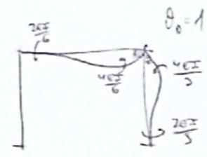
$$(K) = \begin{pmatrix} \theta_a & \theta_c \\ \theta_b & \theta_b \end{pmatrix} = \begin{pmatrix} 4EI(\frac{1}{3} + \frac{1}{6}) & \frac{2EI}{6} \\ \frac{2EI}{6} & 4EI(\frac{1}{3} + \frac{1}{6}) \end{pmatrix} = \begin{pmatrix} 2EI & \frac{EI}{3} \\ \frac{EI}{3} & 2EI \end{pmatrix} = \begin{pmatrix} 20000 & 3333.3 \\ 3333.3 & 20000 \end{pmatrix} = EI \begin{pmatrix} 2 & \frac{1}{3} \\ \frac{1}{3} & 2 \end{pmatrix}$$
