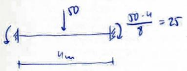
$$\{M\} = \begin{Bmatrix} -25 \\ 25 \end{Bmatrix} \text{ kNm} ; \{\theta\} = (k)^{-1} \{M\} = \begin{Bmatrix} -16 \cdot 10^{-3} \\ 16 \cdot 10^{-3} \end{Bmatrix} \text{ rad}$$
