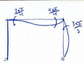
$$(k) = \frac{1}{EI} \begin{pmatrix} \frac{4}{4} + \frac{3}{3} & \frac{2}{4} \\ \frac{2}{4} & \frac{4}{4} + \frac{3}{3} \end{pmatrix} = EI \begin{pmatrix} 2 & \frac{1}{2} \\ \frac{1}{2} & 2 \end{pmatrix} = \begin{pmatrix} 2 \cdot 10^4 & 5 \cdot 10^3 \\ 5 \cdot 10^3 & 2 \cdot 10^4 \end{pmatrix} = 10^3 \begin{pmatrix} 20 & 5 \\ 5 & 20 \end{pmatrix}$$
