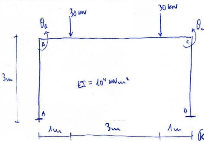
$$(K) = \begin{pmatrix} 4EI\left(\frac{1}{3} + \frac{1}{5}\right) & \frac{2EI}{5} \\ \frac{2EI}{5} & 4EI\left(\frac{1}{3} + \frac{1}{5}\right) \end{pmatrix} = EI \begin{pmatrix} 2\sqrt{3} & 0.4 \\ 0.4 & 2\sqrt{3} \end{pmatrix} = \begin{pmatrix} 21333 & 4000 \\ 4000 & 21333 \end{pmatrix}$$
