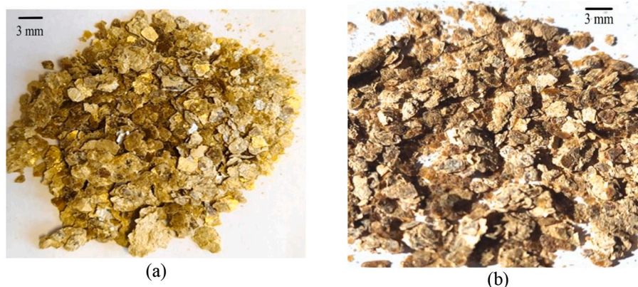
Fig. 4. Appearance of dry vermiculite samples from Uganda (a) and China (b) after hydrothermal treatment.
