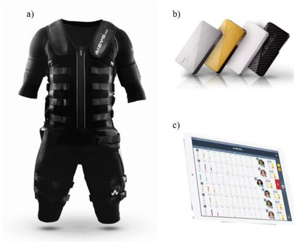
Figure 9. (a) Whole-body electromyostimulation suit; (b) Whole-body electromyostimulation devices that transmit electrical stimuli; (c) Whole-body electromyostimulation app to configure electrical stimuli.
